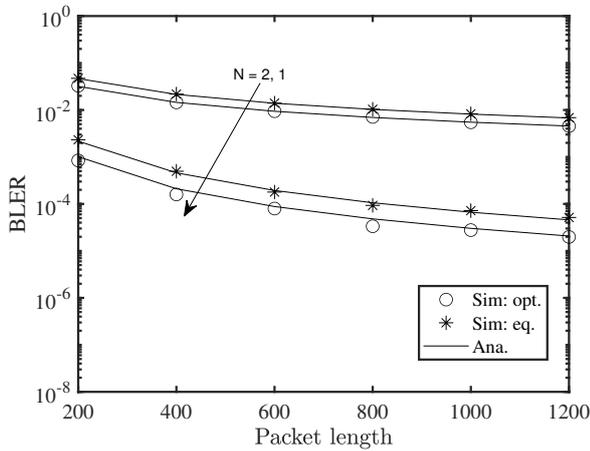
**Fig. 5:** Average BLER versus packet length,  $K = 4$ ,  $N = 3$ .
